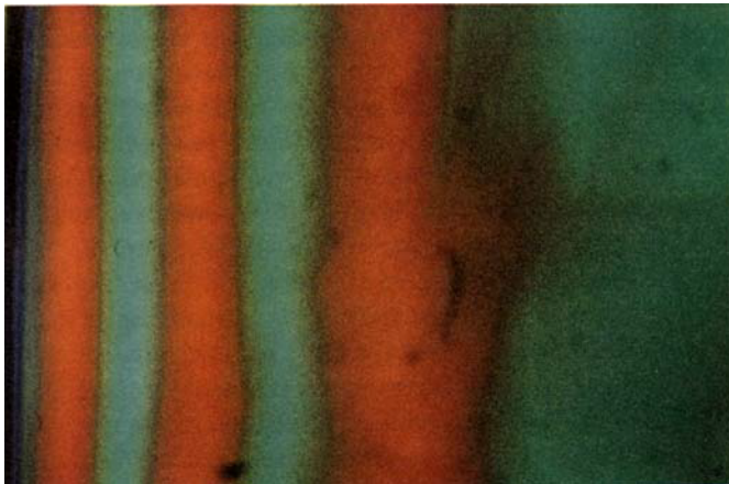
Figure 7. Formation of the striped state from the isotropic state in the smectic C* phase at T = 48^\circ\text{C} ( N = 72 ).
