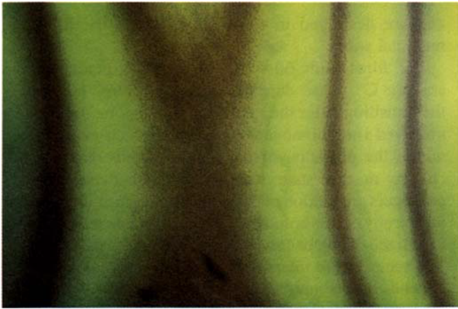
Figure 6. Destruction of the striped state in the middle of the film due to mechanical distortions ( N = 350 ).
