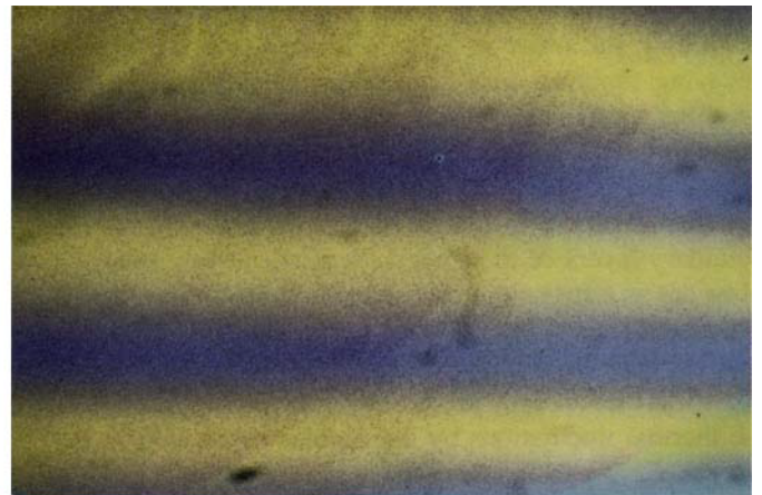
Figure 5. Striped state of the plane director field of the smectic C* phase in the 'bulk' free standing film ( N = 380 ).
